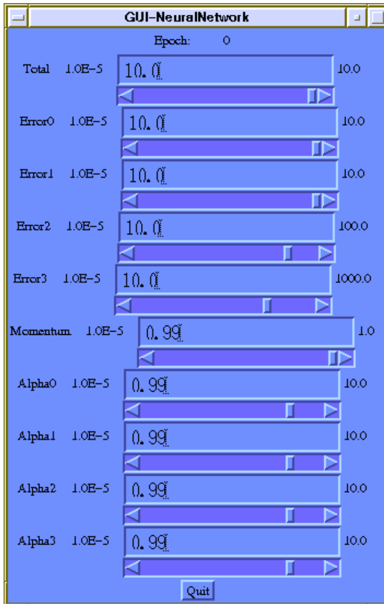
Figure 4.2: Java GUI: The main module of the program communicates with the graphical user interface (GUI) written in Java through CORBA. Users can see the status of the neural network such as the current errors. They can also set the parameters such as learning constants and momentum during learning dynamically by adjusting the slide bar or by typing the number in directly.
